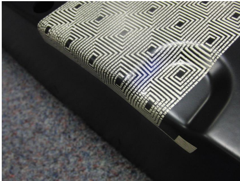
Figure 15 Vacuum form ABS with screen printed silver ink
