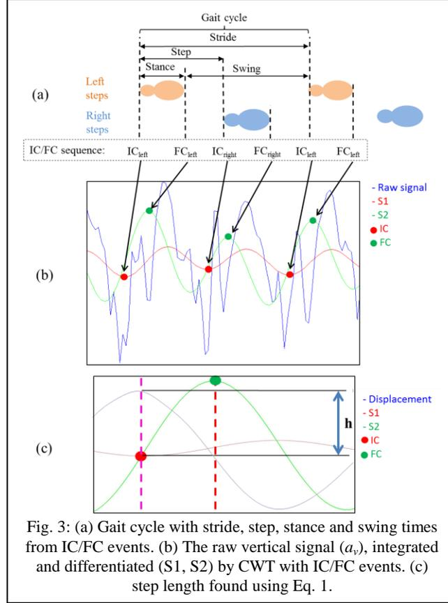
Fig. 3: (a) Gait cycle with stride, step, stance and swing times from IC/FC events. (b) The raw vertical signal ( $a_v$ ), integrated and differentiated (S1, S2) by CWT with IC/FC events. (c) step length found using Eq. 1.
