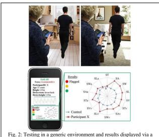
Fig. 2: Testing in a generic environment and results displayed via a web browser with near real time estimation of 14 spatio-temporal gait characteristics (red trace), compared to control data (blue)
