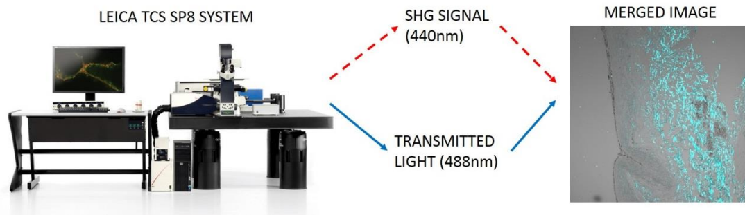
Figure 57 General setup of confocal imaging system used to generate SHG images, showing combination of SHG signal at 440nm with transmitted light at 488nm.
