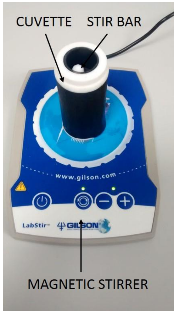
Figure 29 Setup of custom black cuvette on Gilson LabStir containing magnetic stir bar
