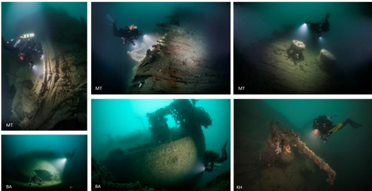
Figure 38: Y Turret teak deck ring; 90 degree snapped deck; identifying capstan and vent at snapped stern section; torpedo salvage hole; stern name lettering; Hotchkiss gun
