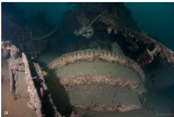
Figure 86: Q Turret shell bogie upper rack
