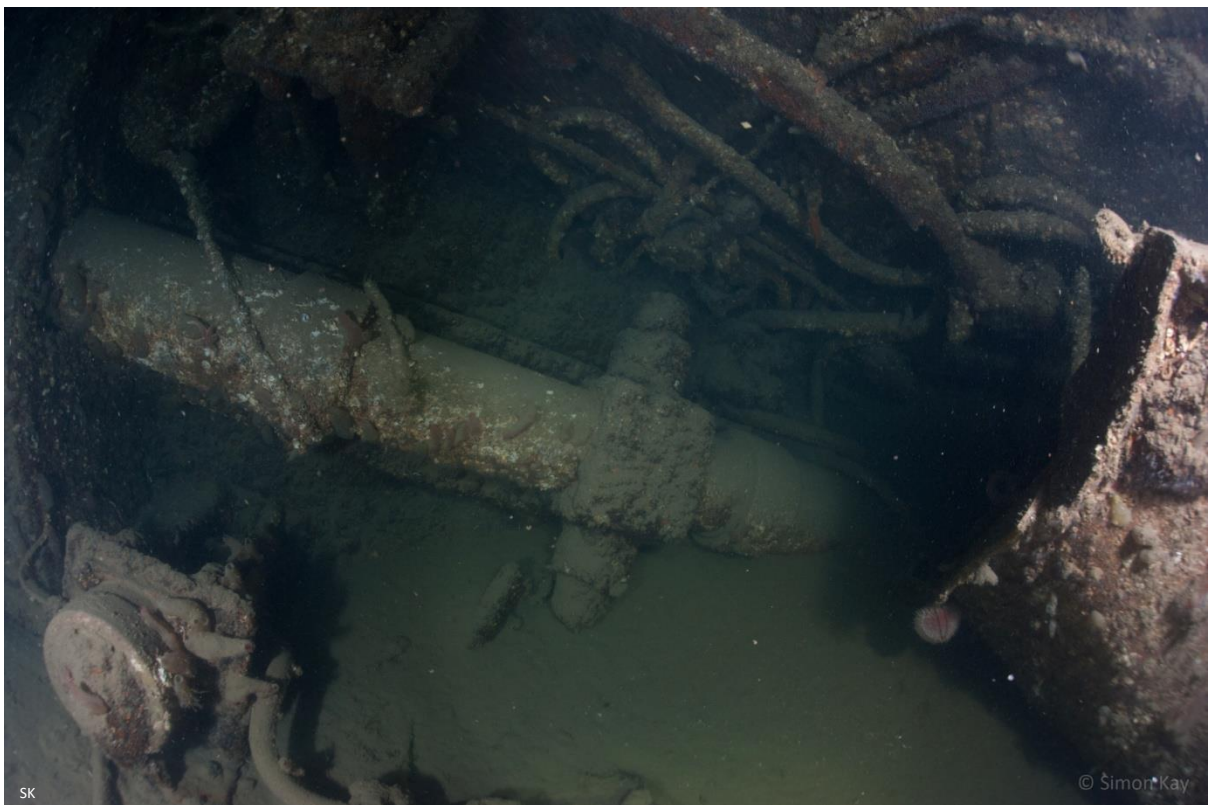
Figure 97: Elevation ram for one of A Turrets guns
