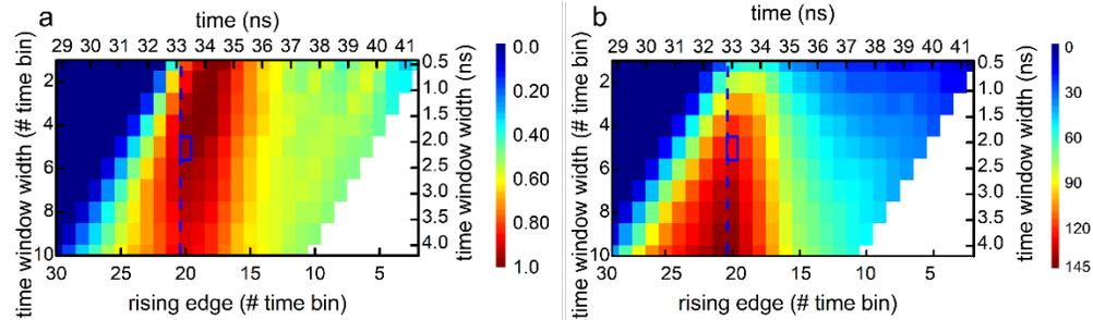
Fig. 5. (a) S/B and (b) S/N plotted against the rising edge of the time window and the width of the time window for the area under the 857 nm SERS peak. The blue vertical dashed line is shown to label the time onset of the signal from the end of the fibre. The blue box shows the chosen timing of bins selected for the other plots in this paper.
