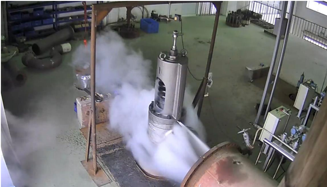
Fig. 3. Photo of a NPMS PRV fully open during performance test.
