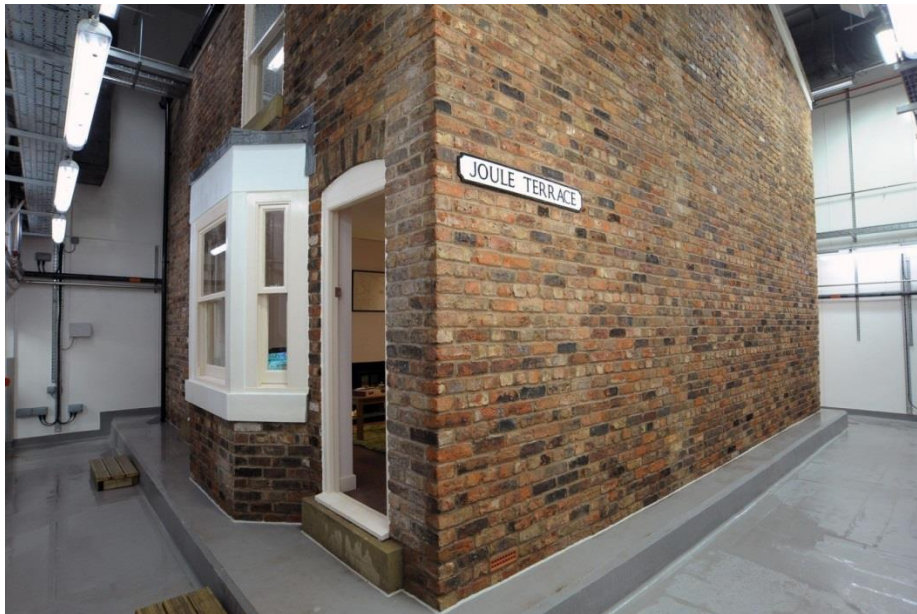
Figure 1: The Salford Energy House within its environmental chamber
