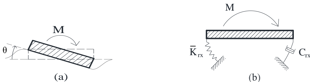
Figure 2. (a) Footing subjected to clockwise moment is rotating towards an angle \theta , (b) Spring-dashpot analogue of the footing rocking mode of vibration
