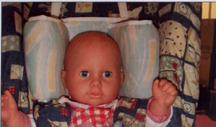
Figure 3.7 Head cushion which limits an infant's head movements during testing
