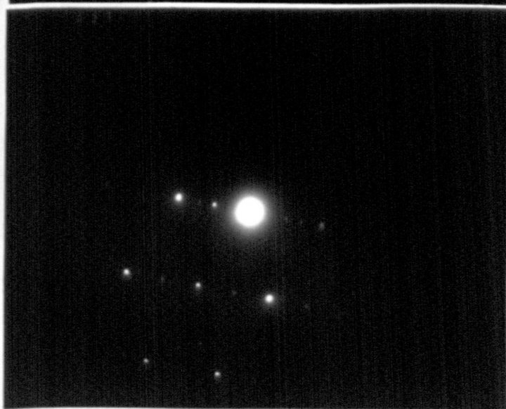
Figure 9.5 Bright field micrograph and electron diffraction patterns of rapidly solidified TiNi ribbon. The patterns b, c, d, e and f are respectively identified as [100]_{B_2} , [113]_{B_2} , [110]_{B_2} , [111]_{B_2} and [120]_{B_2} zones of the CsCl type structure. The patterns corresponding to [110]_{B_2} , [111]_{B_2} and [120]_{B_2} display some extra reflections indicating the presence of more than one phase.
