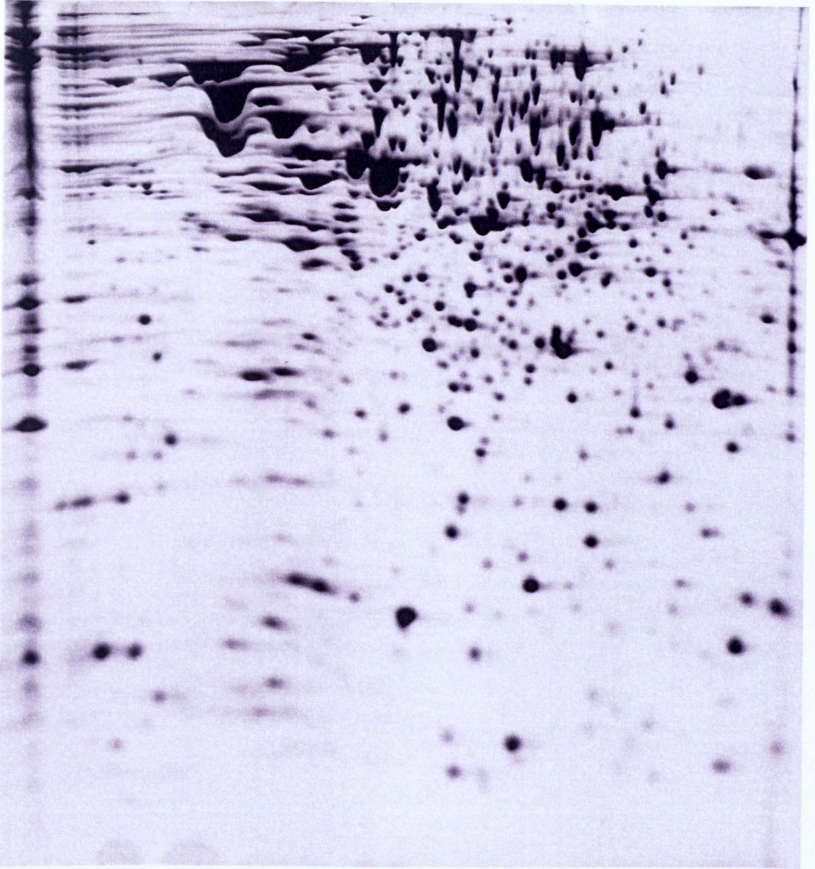
Figure 6.3 2DGE profile of TGC-R \Delta acrB isolate. Total cell extract was separated using pH gradient of 4-7, and 12% polyacrylamide gel. The separated proteins were stained with SYPRO Ruby and visualised using an Ettan Dalt imager (GE Healthcare).
