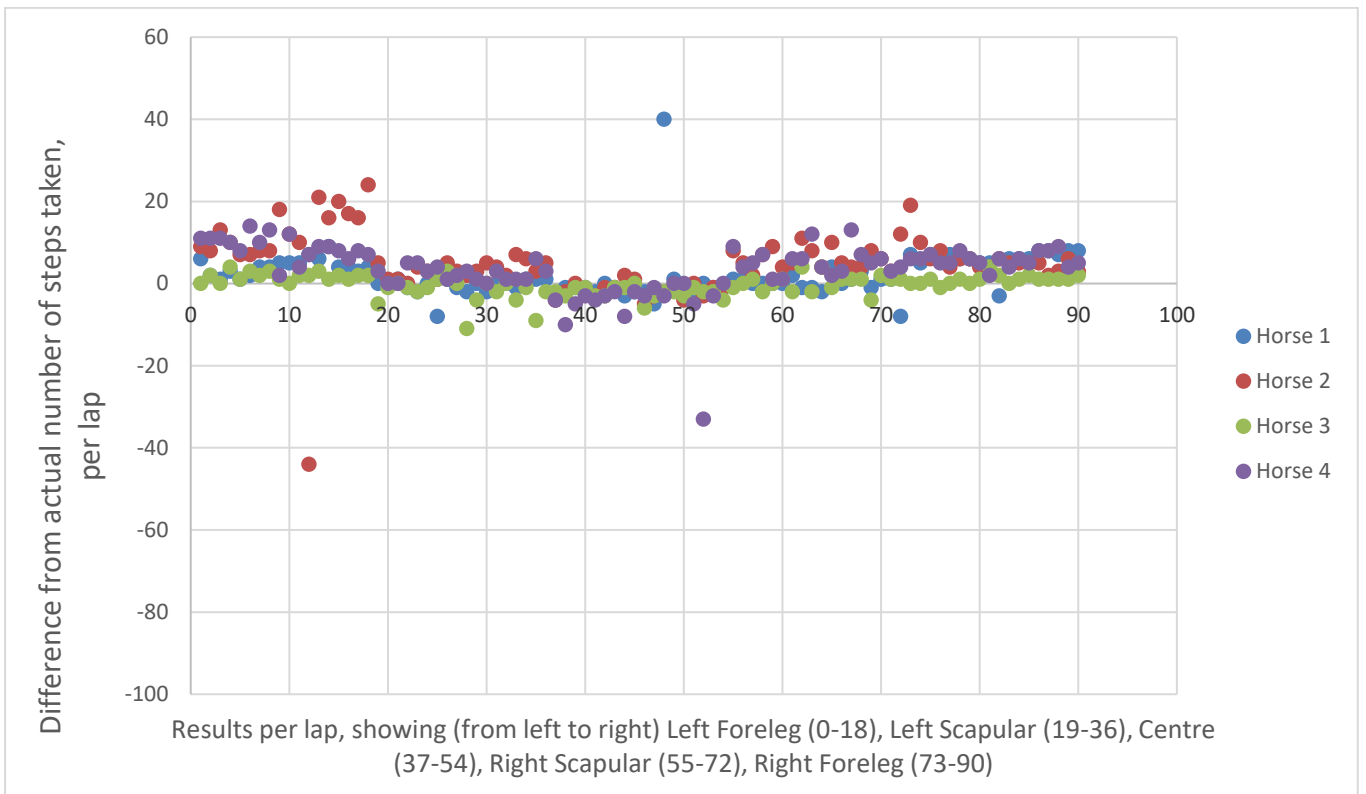
Figure A5.6 Spring lever arm pedometer data distribution compared to actual steps taken by both forelegs in trot per lap
