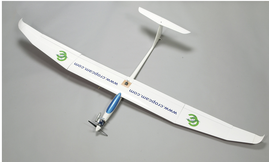
Figure 2.1: Cropcam UAV used for image acquisition over sugarcane fields 1 . ( Cropcam Image 2012 )
