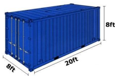
Figura 2 Contêntor standard 20 ft ( http://www.neptunepacific.com/containers.php , 2008)
