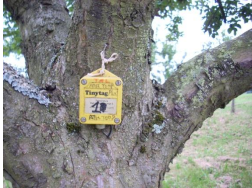
Figure 20 - Temperature data logger, Avel 3, located in the last part of the transect, meadow 5
