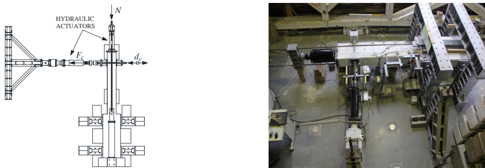
Figure 6. Test setup for column specimens.
