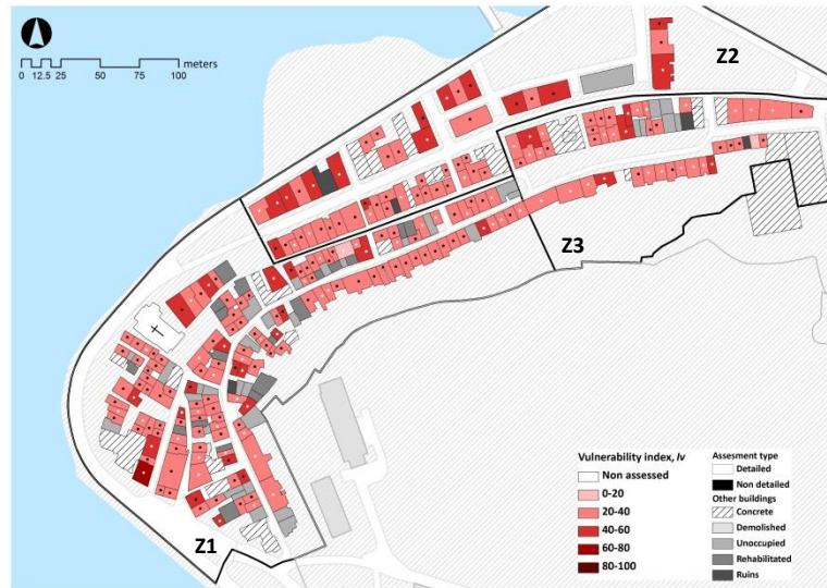
Figure 4. Vulnerability mapping of buildings in zones Z1, Z2 and Z3
