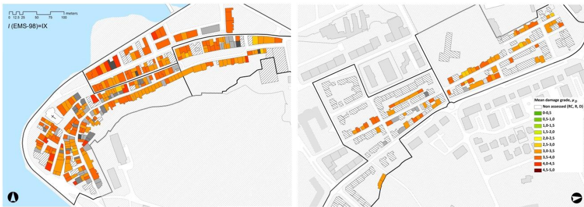
Figure 8. Damage scenario for I(\text{EMS-98})=\text{IX}
