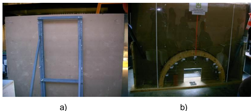
Figure 1 - a) Reaction frame holding the MDF plate; b) Front view of the testing layout with HP Dial Gauges
