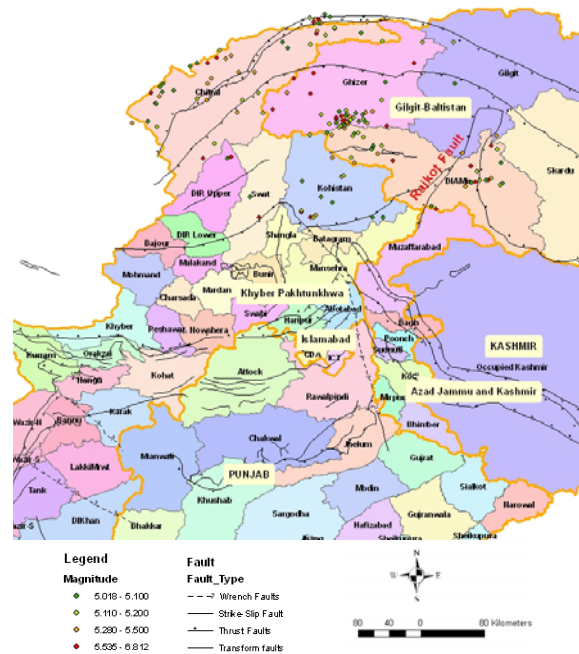
Figure 2.1. Faults and recorded earthquakes around Gilgit-Baltistan
