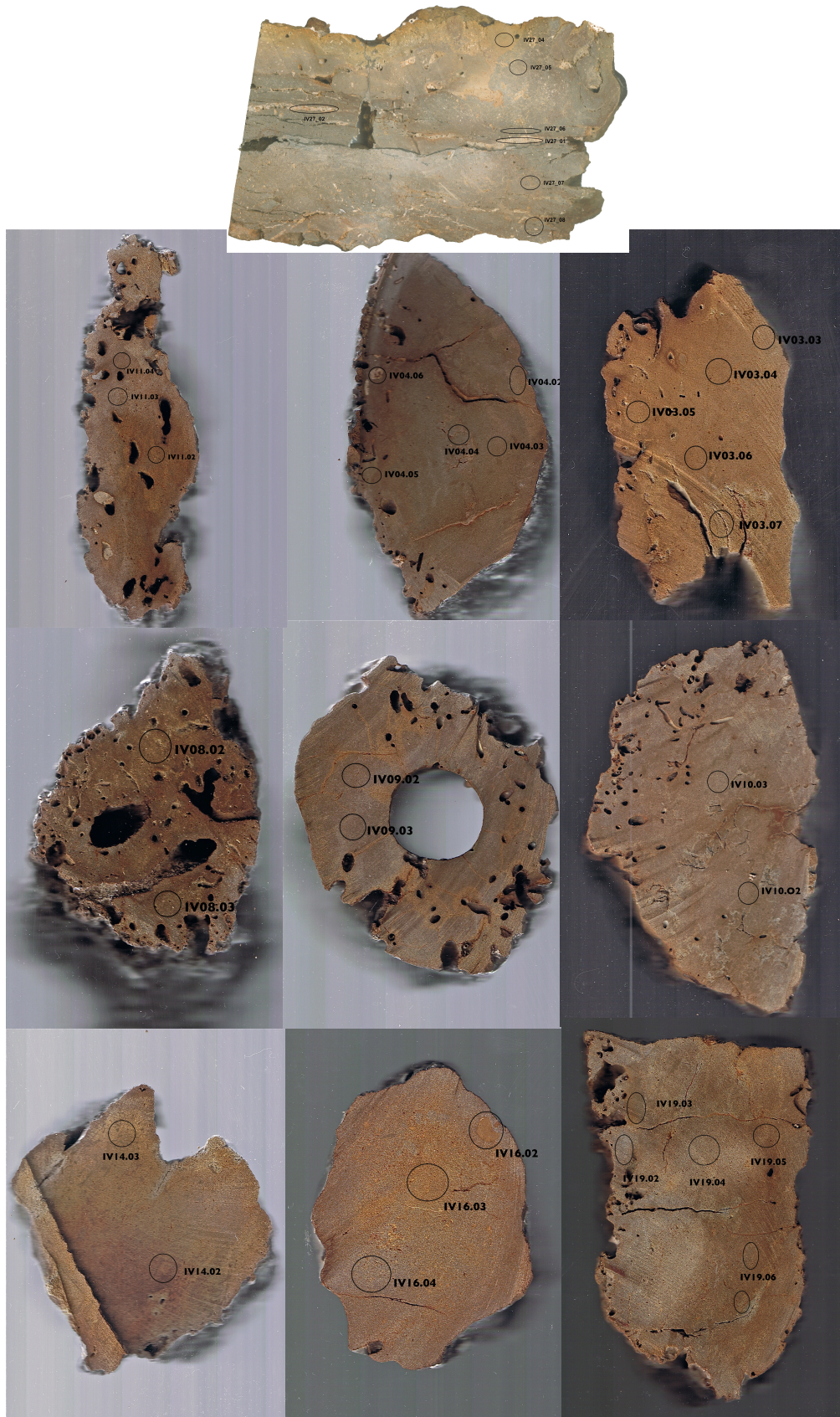
Figure 28: Scans of the sample 600 G and the cutted surface of the chimneys samples. On that have been identify the sub sampling point.
