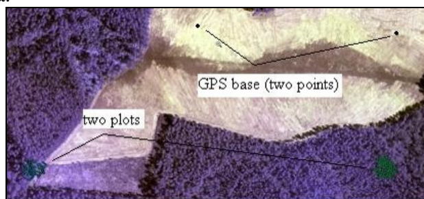
Figure 5: An example of a GPS base to georeference the measurements on two plots.
