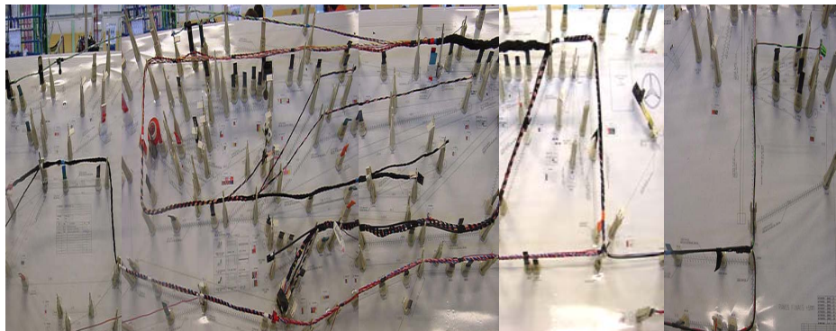
Figure 7.10 – A wire harness assembly jig
