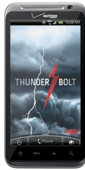
Figure 2.21: HTC ThunderBolt 4G - Verizon Network (US): CDMA 800/1800 MHz EvDO rev.A, LTE 700 MHz.[62]
