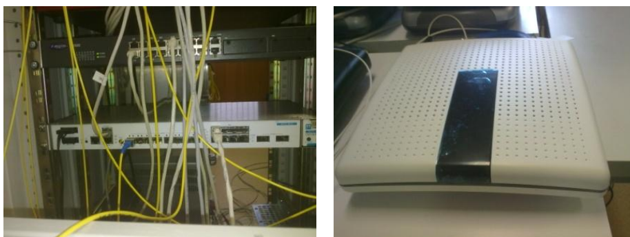
Figure 3.12: (left) OLT- OLT7-8CH (right) ONT7RF1GE
