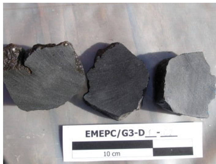
Fig. 4.4 – Picture of a volcanic sample dredge on São Jorge flank. The sample is fresh presenting a dark grey color and small plagioclase phenocrysts were identified (2-3 mm).
