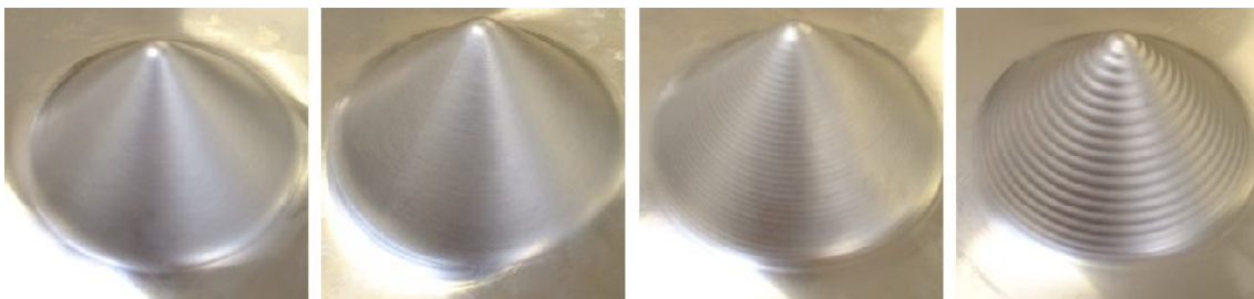
Figure 16 - A cone produced by the Cambridge ISF with varying step sizes. From left to right, 0.2 [mm], 1 [mm], 2 [mm], 4 [mm], [9].
