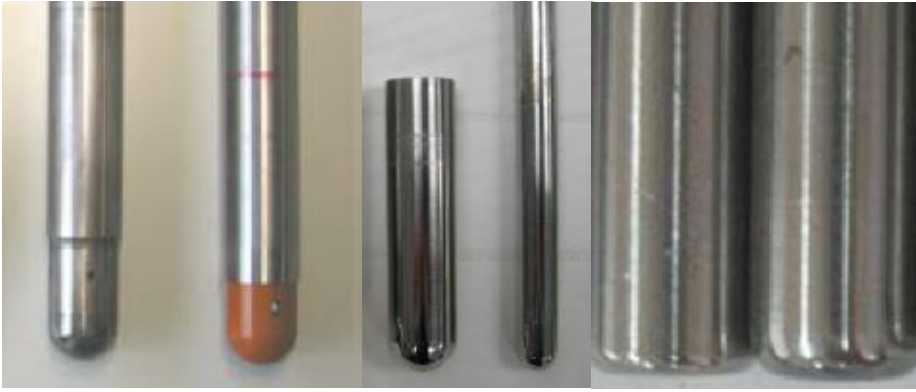
Figure 6 - Coated tools (left), spherical tip tools (center), flat tip tools (right), [2].
