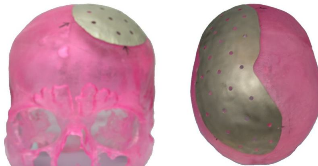
Figure 3 - Cranial implant obtained by incremental forming [6].
