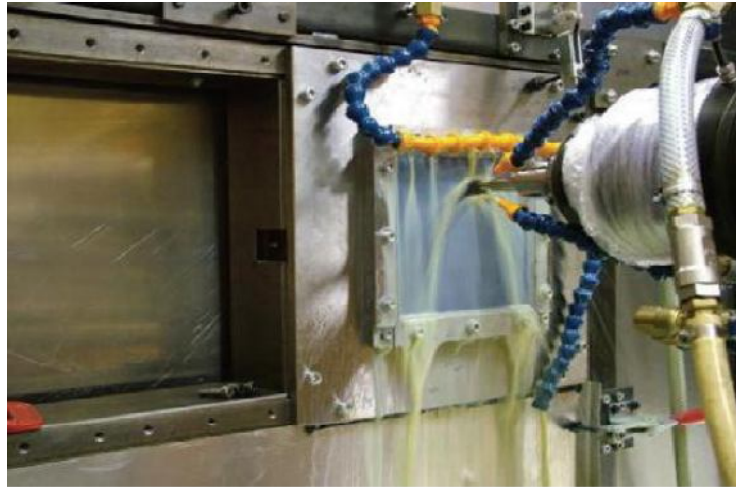
Figure 13 - Robot performing Single Point Incremental Forming [6].
