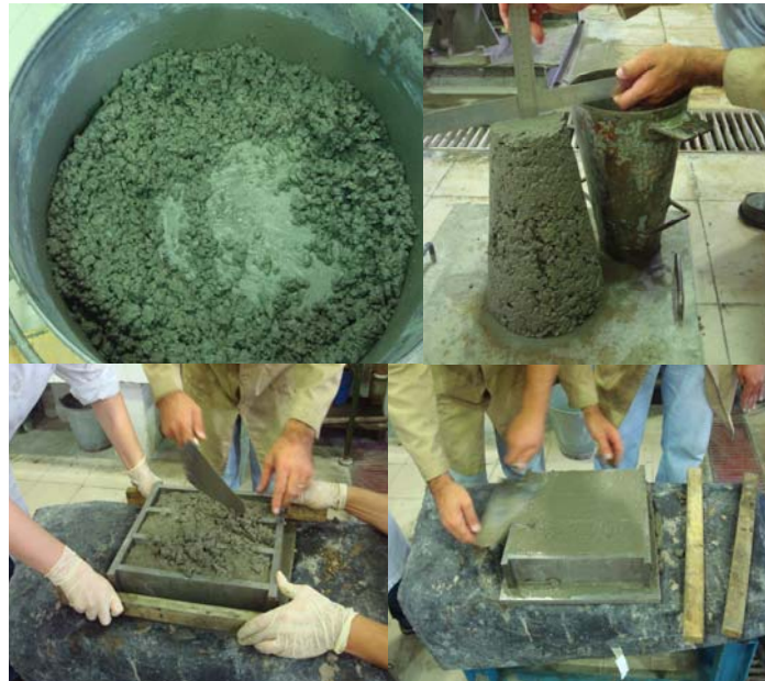
Figure 5.5: Preparation of Concrete prisms for ASR concrete test methods.
