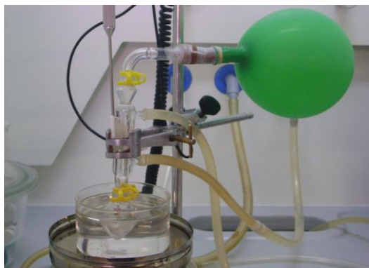
Figure 5.1: Lab setup for the preparation of Silica@APS.
