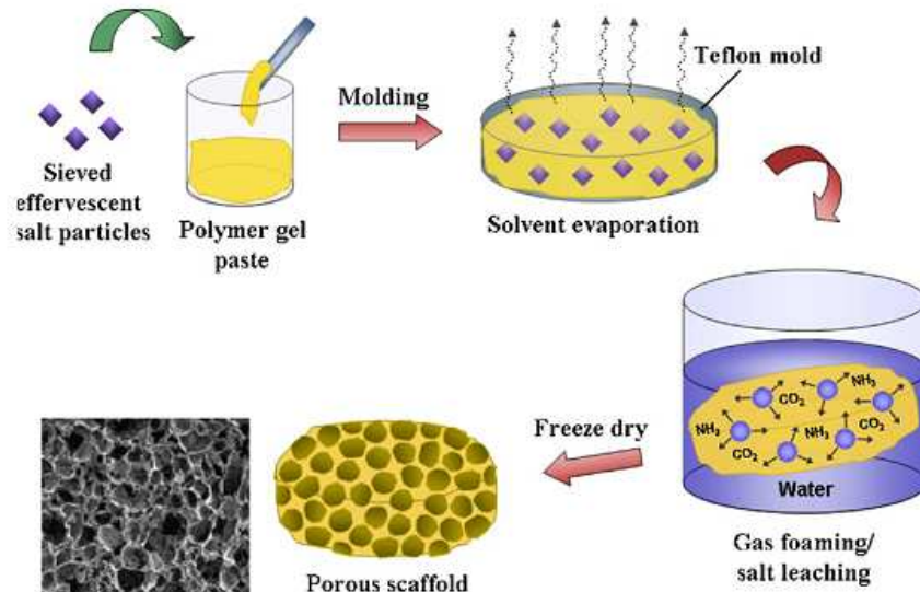
Figure 2-11 Illustration on scaffold manufacturing using particle leaching method 50
