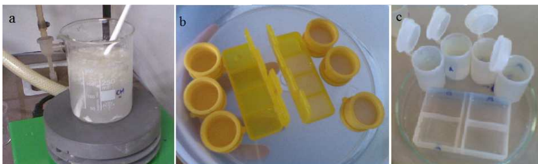
Figure 4-4 (a) Chitosan Solution Preparation with Magnetic Stirrer; (b) and (c) Differently shaped containers used for preparing the chitosan-based scaffolds
