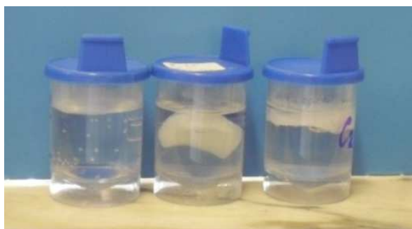
Figure 4-10 Samples for bioactivity test in SBF: blank SBF (left), chitosan/chitosan composite scaffold (middle and right)
