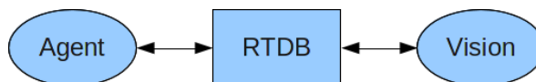
Figure 4.4: Architecture for communication between the agent and the vision using the Real-Time Data Base (RTDB).
