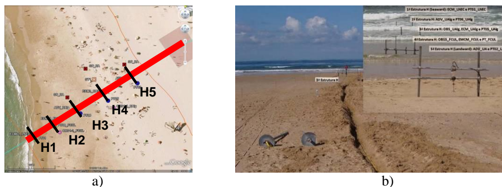
Fig. 3 – a) Location of the beach profile where the instruments were positioned (Google Earth) and b) Beach profile and location of the H-structures used in the field campaign (Bezerra and Ferreira, 2010).
