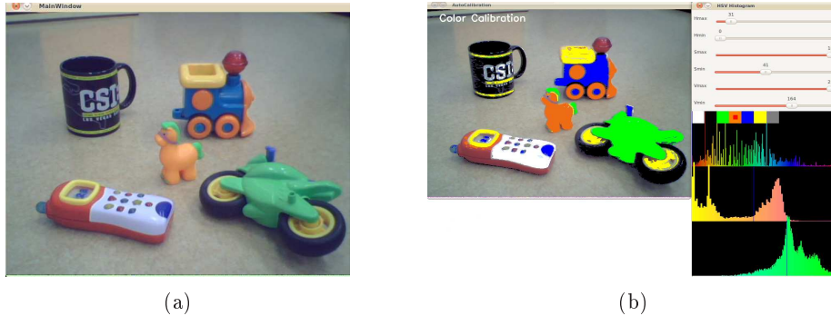
Figure 3.6: On the left, an original image acquired by the NAO camera and displayed by the NaoViewer application. On the right, the same image with the colors of interest classified by means of the NaoCalib application.
