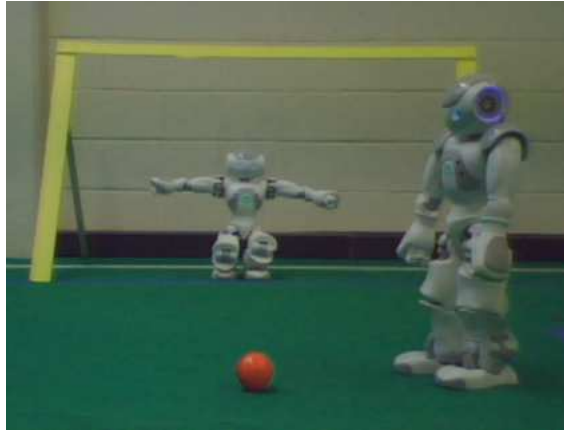
Figure 1.2: An example of an image acquired by the NAO camera during a game, representing what the robot “sees”.
