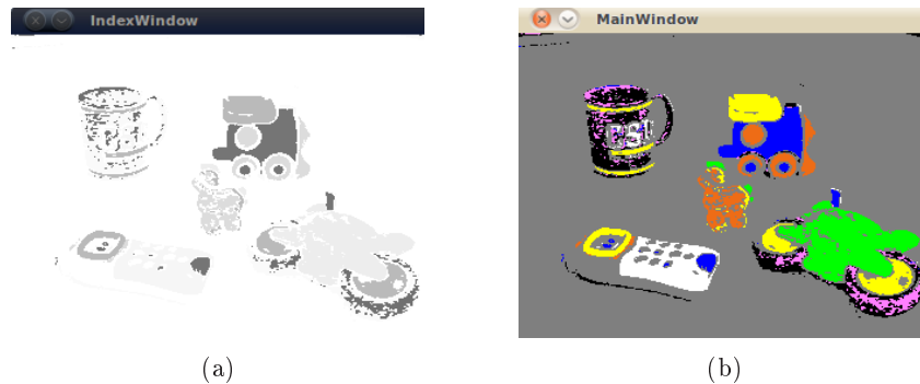
Figure 3.7: On the left, the index image with all the classified colors labeled. On the right, the RGB image obtained by “painting” the index image according to the labels.
