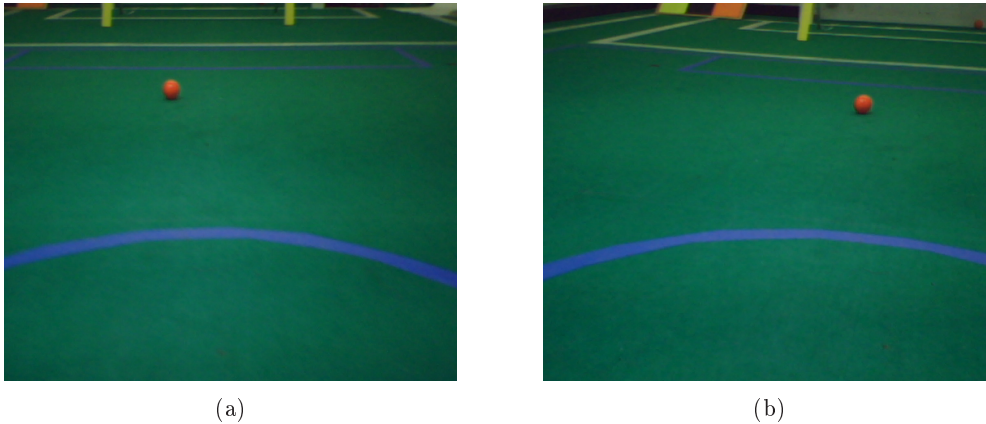
Figure 1.3: Two consecutive frames acquired while the robot is moving. Due to its locomotion, consecutive frames acquired by the camera of the robot might represent different views of the surrounding world.
