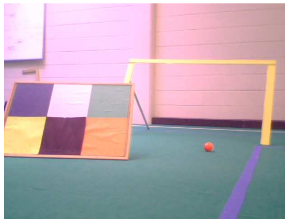
Figure 4.11: An example of an image acquired with the camera working in auto-mode. The color of the carpet is different than the green we would expect to see and the white areas and the yellow goals are too bright.
