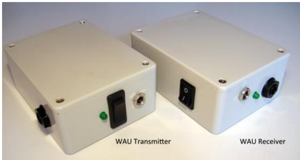
Figure 48: Final assembly of Wireless Audio Unit
