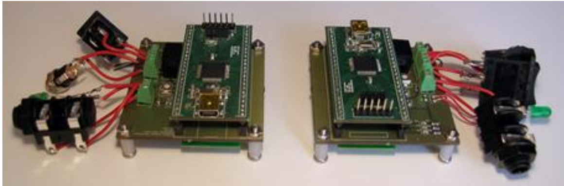
Figure 47: Produced PCBs of Wireless Audio Unit
