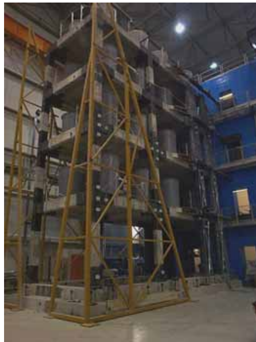
Figure 8. Earthquake tests at ELSA. Experimental set-up
