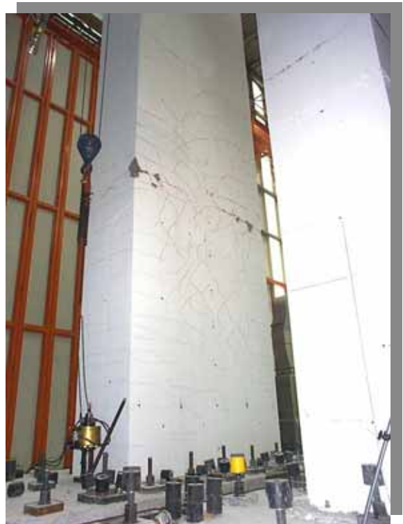
Figure 2. Bridge pier model (scale 1:2.5 - hollow box cross-section) of an existing highway-bridge in Austria tested at ELSA. Failure at 3.5 m from the base (Pinto & Tsionis 2001, Flesch et al. 2000)
