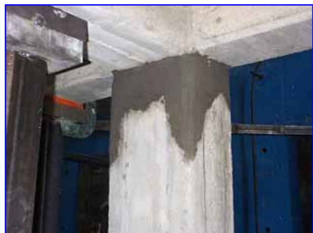
Figure 14. Failure (shear-out) of the column/joint interface: Schematic representation (left), photographic documentation (right)
