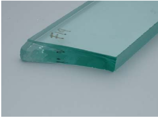
Figure 6: Crack pattern of float glass.
