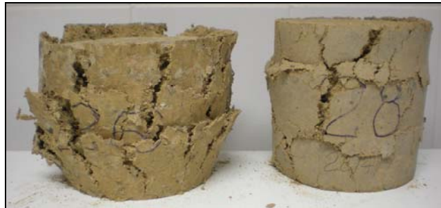
Figure 4: Kraftterra samples after compression tests for different compactation humidity contents: 21% (left) and 13% (right).
