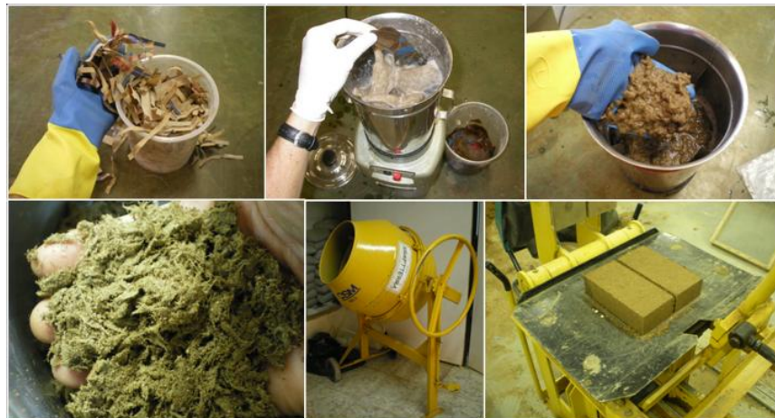
Figure 1: Kraftterra blocks production: cement bags cutting; fibres dispersion; mixture with soil-cement; compressed blocks.
