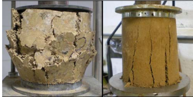
Figure 3: Kraftterra (left) and Soil-cement (right) samples after compression tests.
