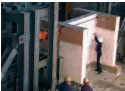
a) Cyclic test (Blondet et al. , 2005)
