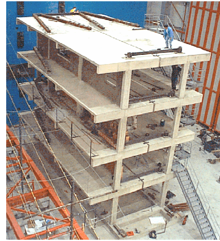
Figure 1. Tested frames: a) elevation views of the frames; b) models in the ELSA laboratory
