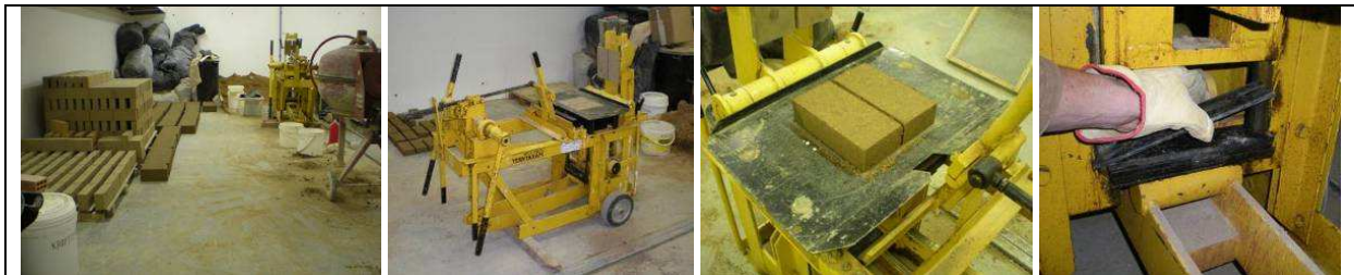
Figure 3: Press TERSTARAM. Detail of the height adjust system of the form (right).
