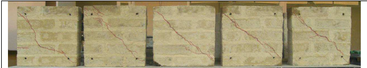
Figure 7: Prisms at the end of the diagonal compression tests. The fissure lines were highlighted.
