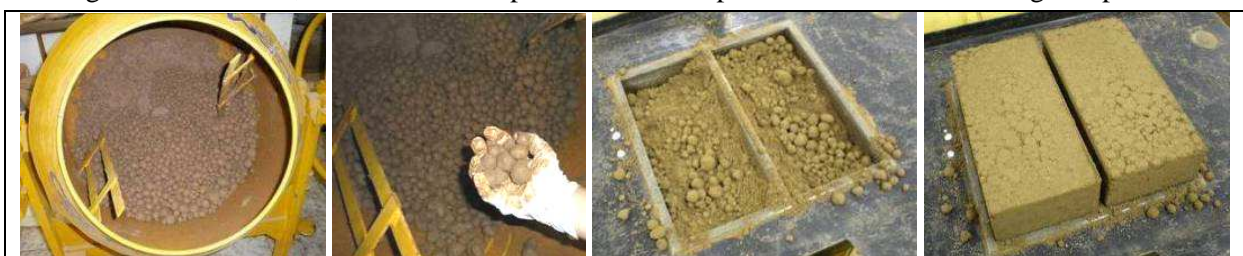
Figure 2: Mixture of Kraftterra in a concrete mixer resulting in clusters
