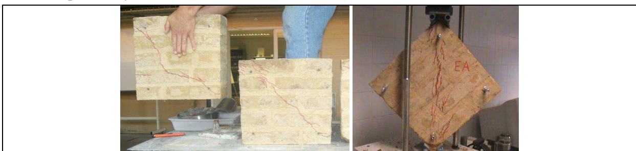
Figure 8: Prisms when lifted show bond strength in the rupture area (left), and Kraftterra prism that went through accelerated aging cycles - appearance after the test (right).
