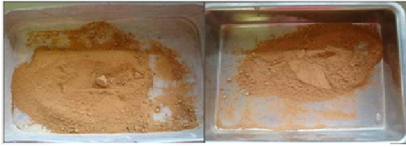
Fig.6 - Some mortar samples for the granulometric analysis
