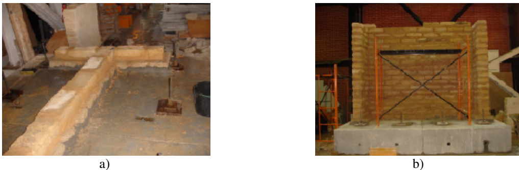
Figure 2.1. Adobe wall construction: a) beginning of the construction; b) final phase of the construction (before plastering)
