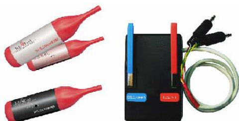
Figure 5. IntergraMouse (top-left), IntegraSwitch (bottom-left) and wheelchair command (right) interfaces
