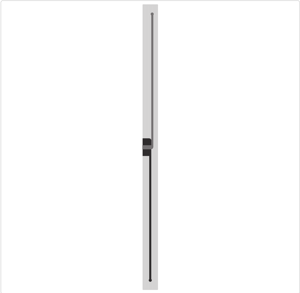
Figure 3.2: Proposed dipole-based PCB antenna designed for use with the sensor node, shown on a 1:1 scale (the rectangular area represents the substrate and the other two structures correspond to the arms of the dipole, with the upper arm being on the top side of the substrate and the lower arm being on the bottom side).
