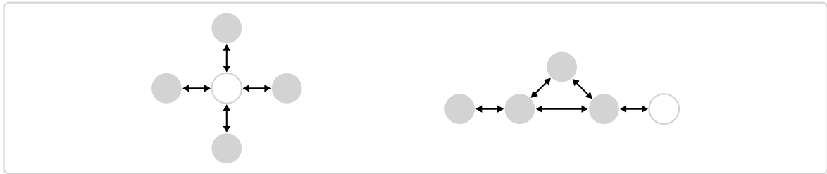
Figure 1.1: Star and mesh network topologies, represented on the left and right sides of the figure, respectively (in both network configurations, the empty circles represent sink nodes whereas the filled circles correspond to ordinary sensor nodes).
