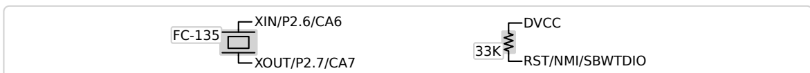
Figure 3.7: Other hardware components integrated into the sensor node, which, from left to right correspond to a crystal oscillator and a to a single resistor.
