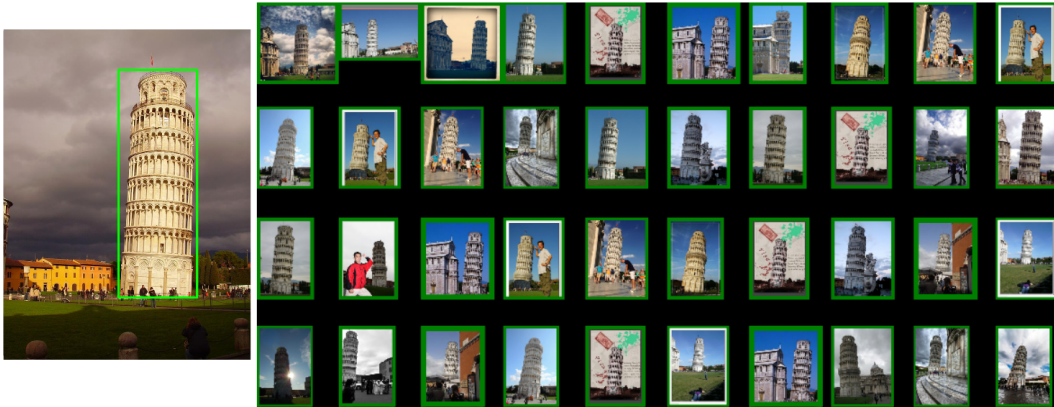
Figure 6.6: The top-10 ranked results for query 766 of the INSTRE dataset. Sum-pooling aggregation is used as feature encoding. The first row contains of unweighted features (AP = 0.805); the second, Gaussian weighted features (AP = 0.774); the third, L^2 -norm weighted features (AP = 0.806); and last saliency weighted features (AP = 0.744).
