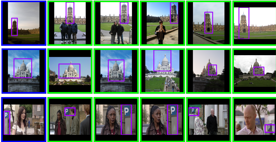
Figure 4.7: Examples of the top-ranked images and localizations based on local CNN features encoded with BoW. Top row: Christ Church from the Oxford Buildings dataset; middle row: Sacre Coeur from Paris Buildings; bottom row: query 9098 (a parking sign) from TRECVID INS 2013.
