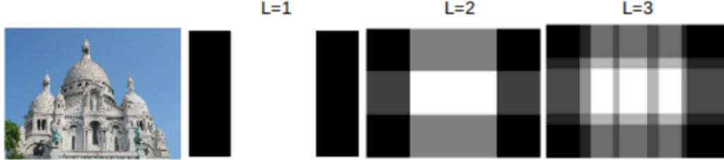
Figure 6.2: Weighted maps \alpha(i, j) obtained from the sliding-window strategy applied in R-MAC at three different scales L .
