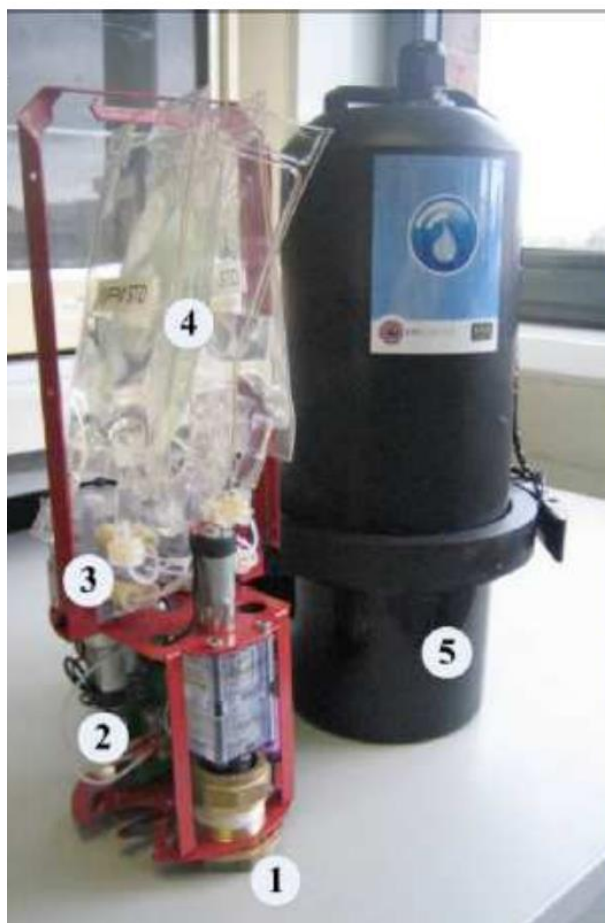
Fig. 1.13. The second generation phosphate sensor. (1) Sample inlet (2) control board, detection system (3) peristaltic pumps (4) reagent bags and (5) enclosure. 43
