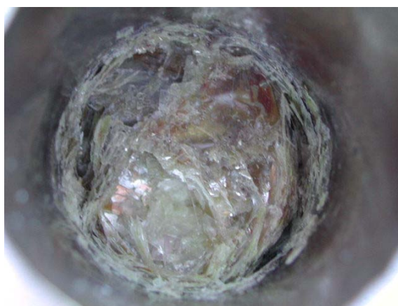
Figure 3.1 Solidified mass of \text{SrBi}_2\text{Ta}_2\text{O}_9 crystals and flux inside the Pt crucible (2 cm base diameter) after the growth experiment using thermal profile TP3.
