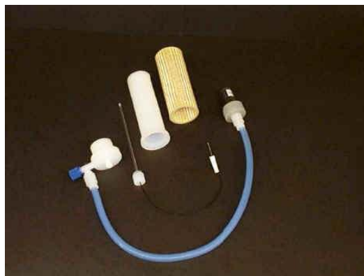
Figure 1.6- Reaction vessel of a microwave heating apparatus, CEM Mars 5 Microwave Accelerated Reaction System. From left to right there are the vessel lid with the pressure release valve, the temperature sensor (sapphire or glass tube with optic fiber temperature sensor inside), the Teflon reaction vessel, the Kevlar explosion proof sleeve and the pressure transducer (attached to the pressure valve) [19] .
