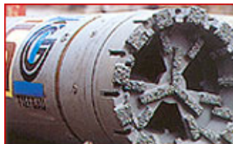
Figura 18. Pipe eating : pormenor do escudo microtunneling [30]
