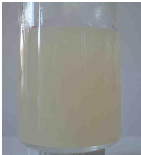
Figure 7.2.26. Optical photograph of the sol-gel formulation doped with cerium molybdate nanoparticles.
