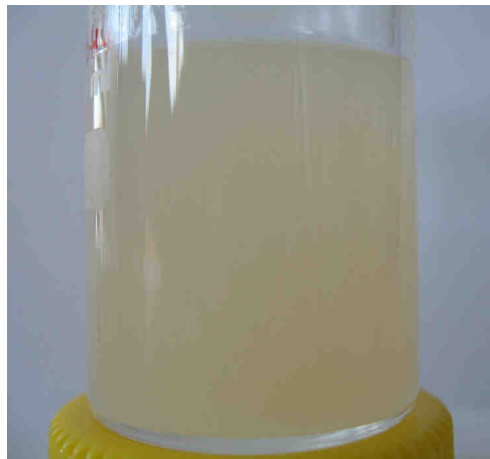
Figure 7.2.21. Optical photograph of the sol-gel formulation doped with halloysites.
