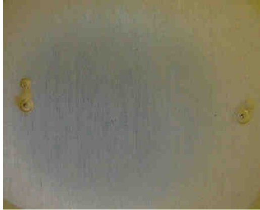
Figure 5.1.9. Optical photograph of the surface of the AA2024 at the beginning of the immersion test in NaCl solution; on the left and right sides bubbles are seen.
